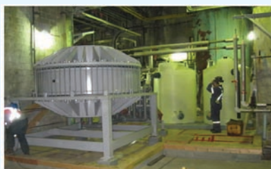
10 This GAP system was recently installed in a western Canadian Kraft pulp mill for the recovery of sulphuric acid from chlorine dioxide generator effluent.
