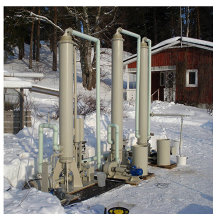
26 Test run with pilot stripping and liquid redox plant.
