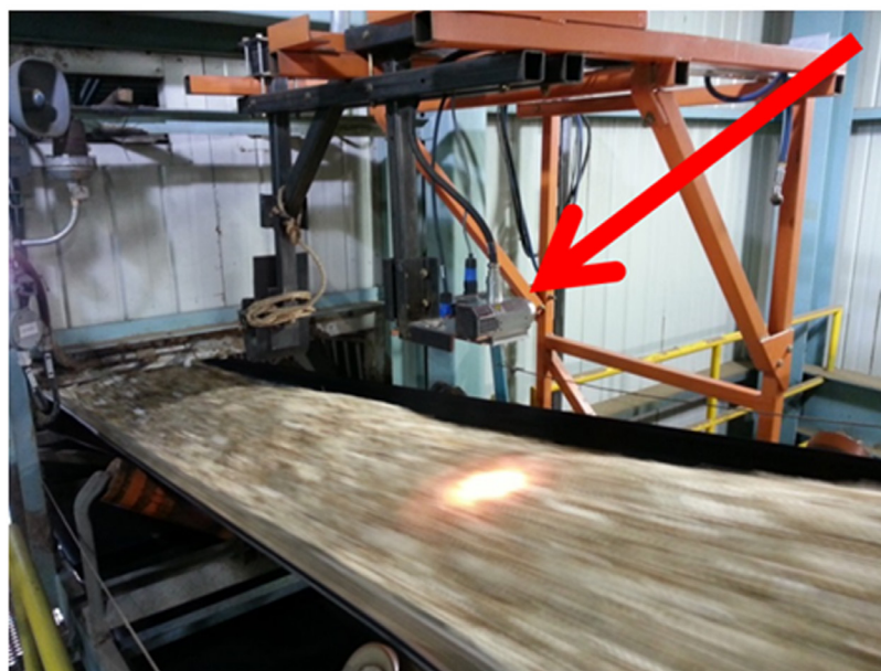
7 Sensor head installed over the chip conveyor belt at the mill.
