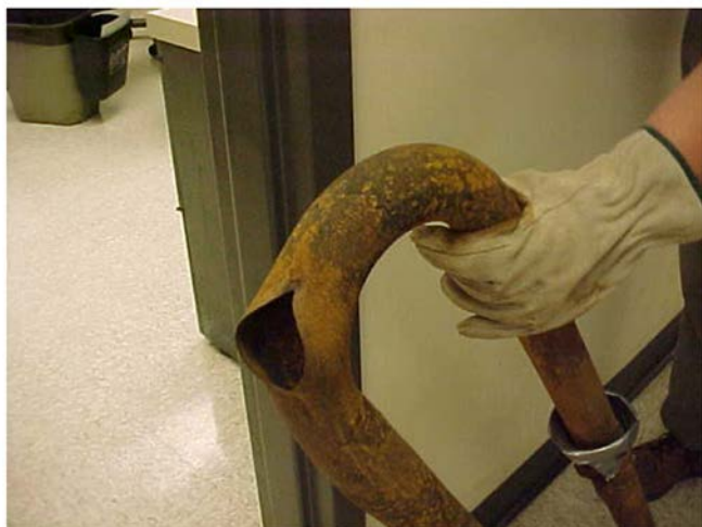
46 Short-term overheat failure of superheater tube.
