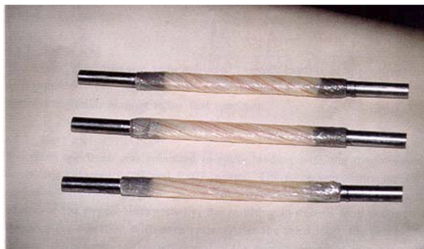
32 Fibreglass “fibres” with fibril angles of 10°, 20°, and 30° [9].
