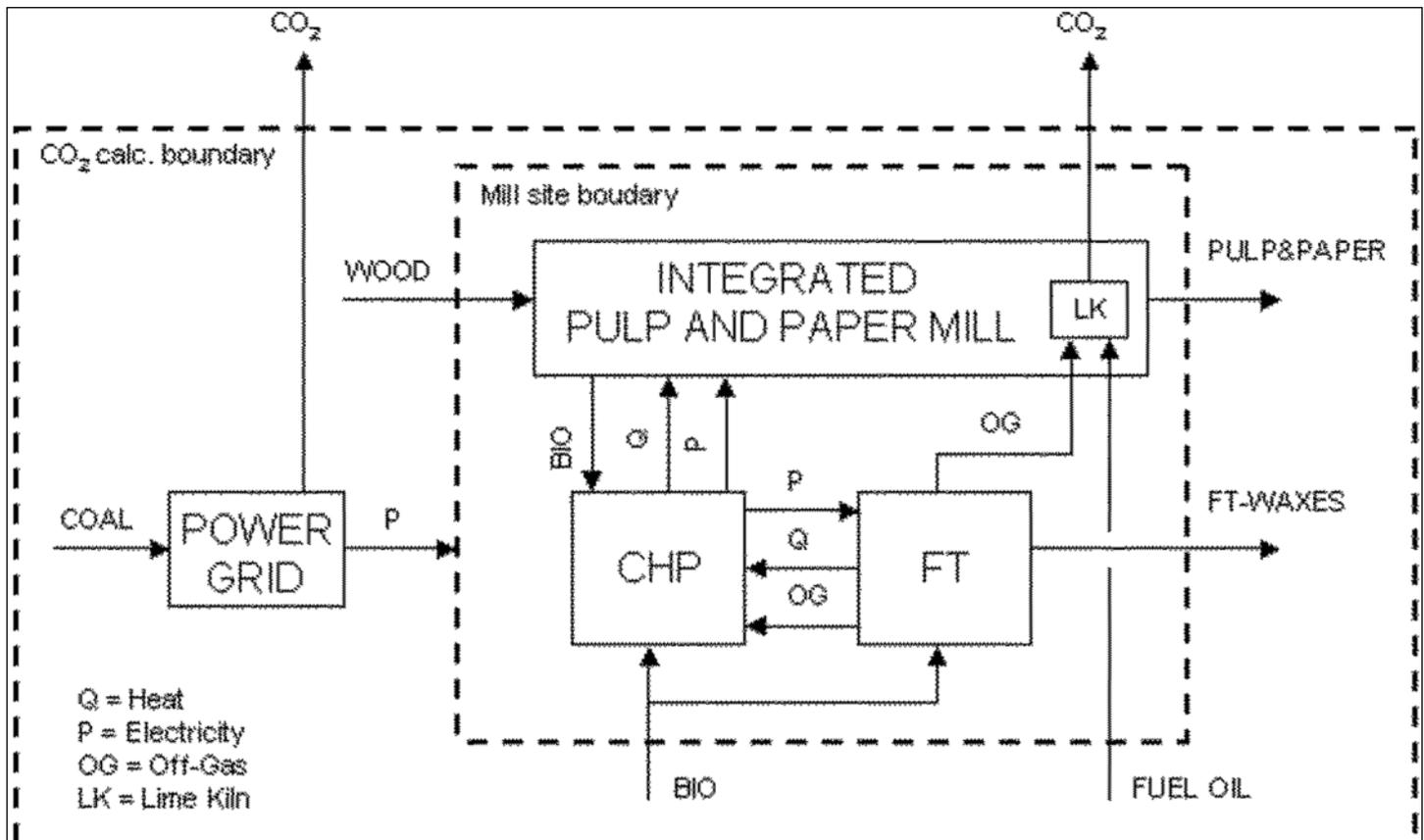
Fig. 2 - Mill-site boundary and CO<sub>2</sub> calculation boundary.
