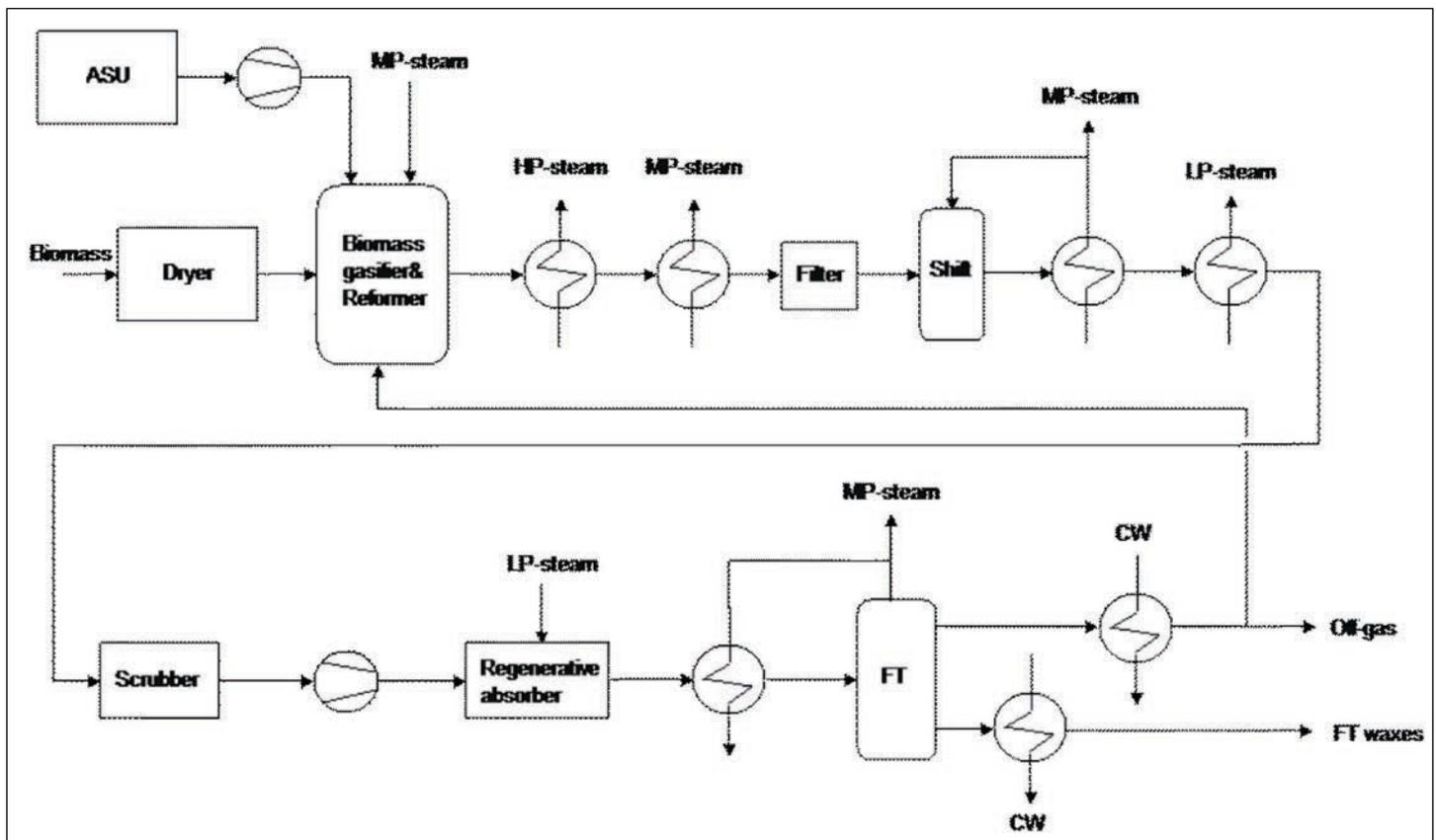
Fig. 1 - Flow-sheet of the Fischer-Tropsch process.
